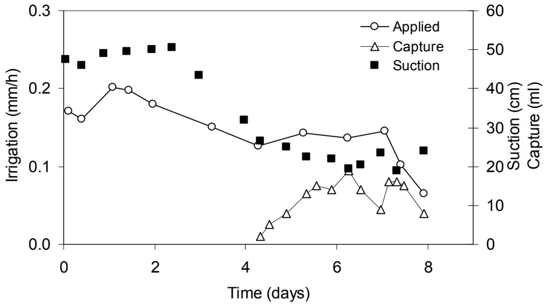
Fig. 3. The rate of drip irrigation applied to the drum, the capture rate of water in the WFD and the soil suction at the depth of measurement of the WFD.
