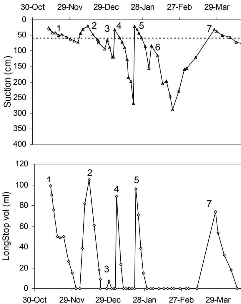
Fig. 4. The soil suction in the 'wick' of the LongStop (top) and the volume of water in the LongStop (bottom). The horizontal dotted line in the top graph demarks the theoretical sensitivity limit of the LongStop, above which the WFD should contain water. The numbers refer to the seven irrigation or rainfall events.
